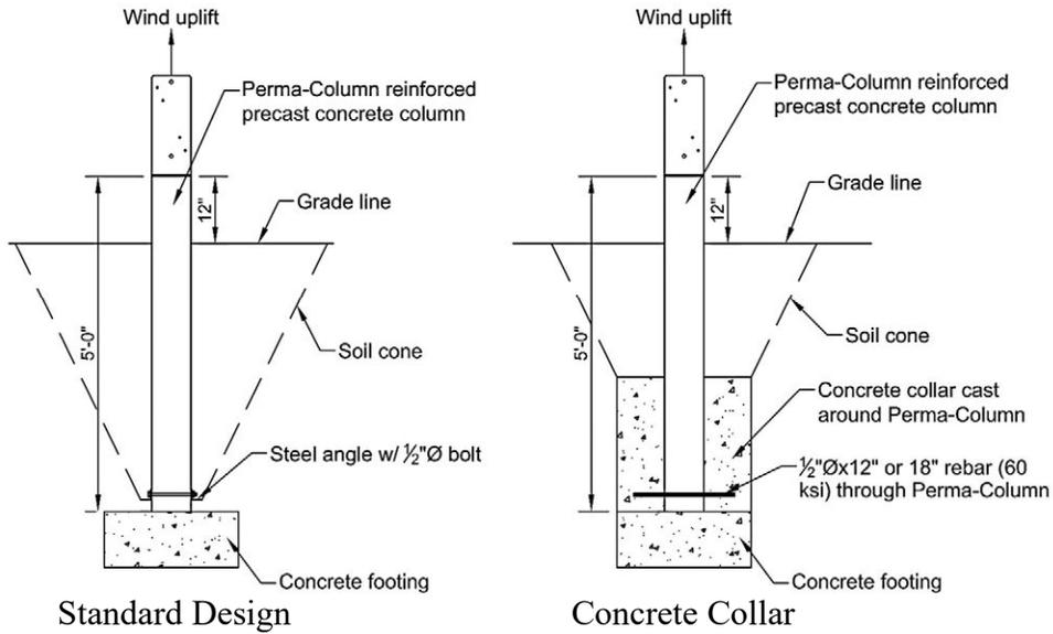
**Figure 11.1: Standard Foundation and Foundation with Concrete Collar**
